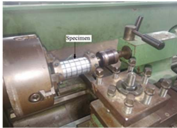
Figure 1: Specimen mounted on the fixtures using the lathe machine.
