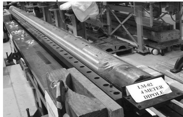
Fig. 1. 4-m long Nb 3 Sn RRP coil.
