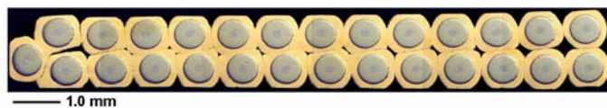
Fig. 3. Cross-section of a key-stoned F3 Nb 3 Al Rutherford cable with a high compaction factor 87.2 %. 14.2 mm x 1.78 mm average.
