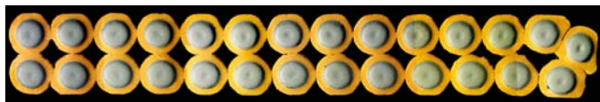
Fig. 2. Cross-section of a rectangular F1 Nb 3 Al Rutherford cable with a low compaction factor 82.5 %. 14.2 mm x 2.0 mm.
