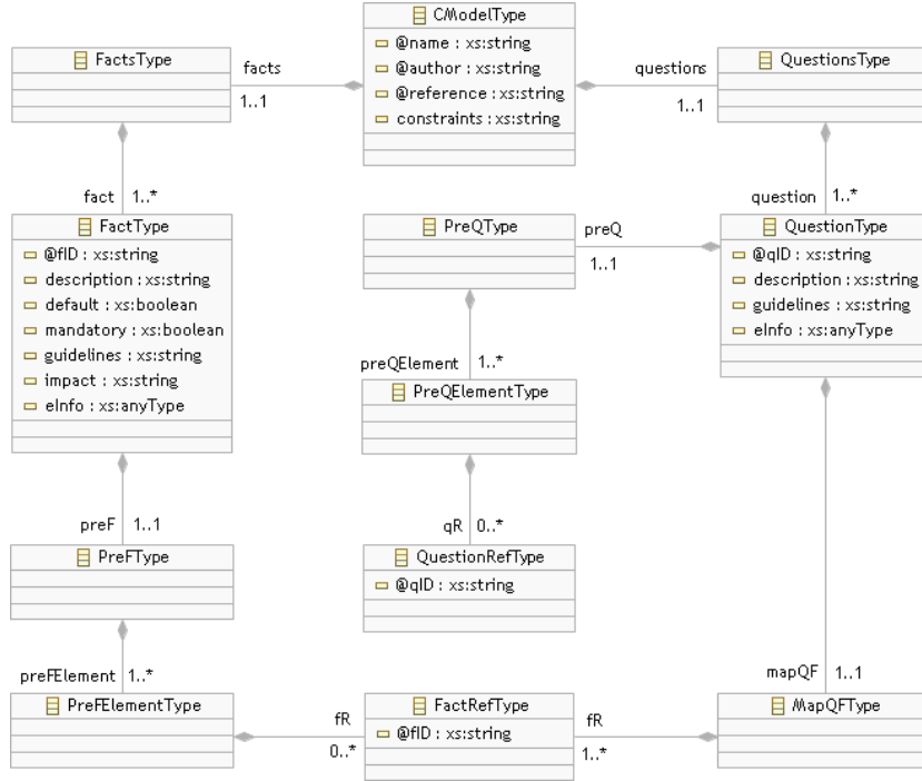
Fig. 7. The UML representation of the XML schema for the input file.
