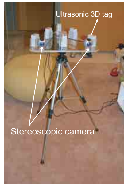
Figure 19. Ultravision (stereoscopic camera with ultrasonic tags) for creating simplified 3D shape models
