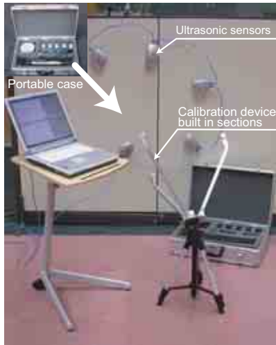
Figure 18. Portable ultrasonic tagging system
