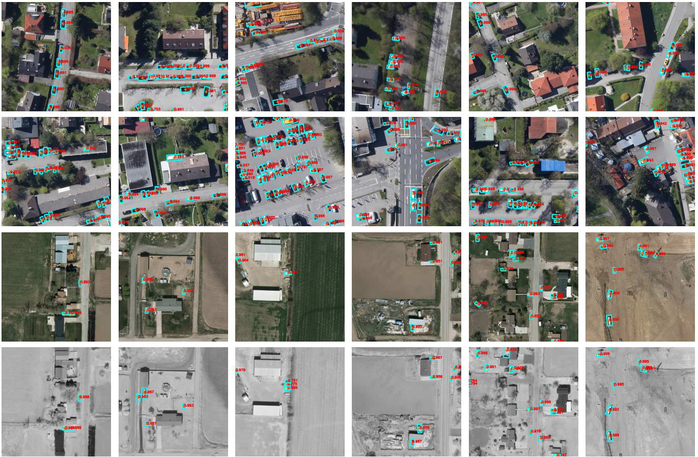
Fig. 8. Examples of multioriented vehicle detection of the proposed method. First two rows: test samples in DLR 3K Munich Data set. Last two rows: test samples of VEDAI Data set (two image modes: RGB and NIR). Best viewed zoomed in.
