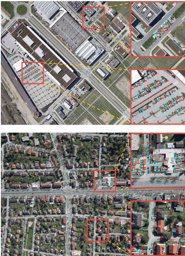
Fig. 1. Examples of multioriented vehicle detection produced with the proposed network, over two scenes taken from DLR 3K Munich Data set. Best viewed zoomed in.
