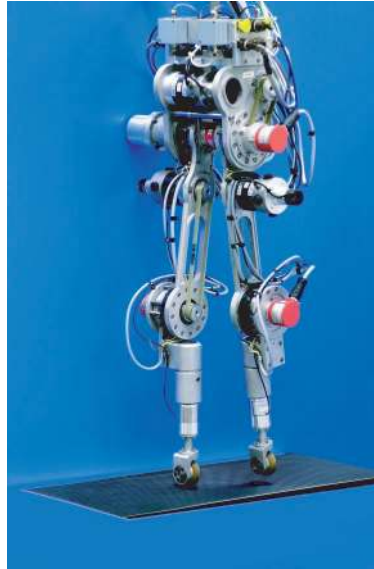
Fig. 1. Photo of RABBIT. The robot was designed to facilitate the development of theoretically-sound control algorithms for walking, running and balancing.
