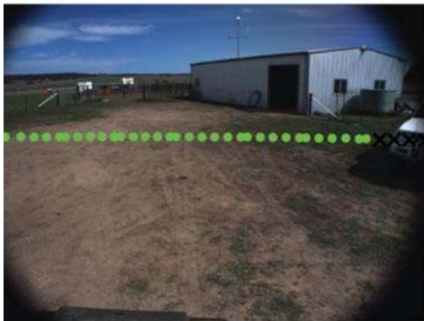
Figure 15. Results obtained from the RGS system in the presence of a large obstacle to the right: output of the RGS system (a); results overlaid on the camera image (b) and on the laser-generated ground-truth map (c).
