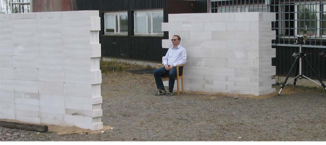
Fig. 1. Setup of (right) radar antennas, a human target, and concrete wall sections.
