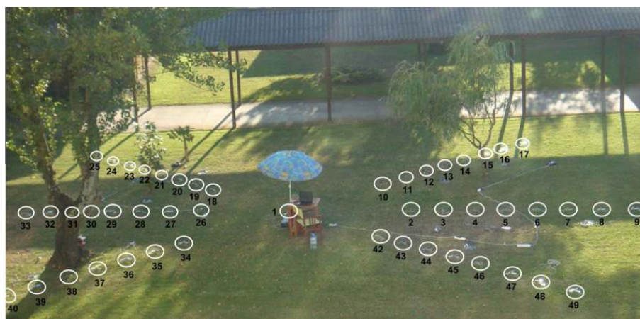
Fig. 4. Nodes distribution according the radial topology, at an outdoor environment (circles were added to the picture to identify nodes positions).
