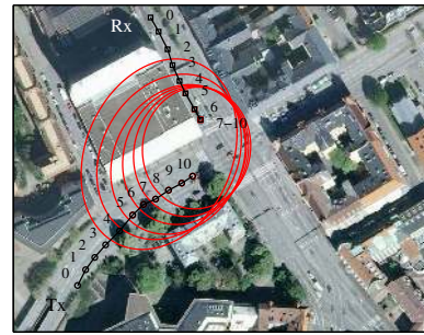
Fig. 7. Scattering ellipses for the first arriving discrete MPC before LOS is obtained in Fig. 6. The markers indicate the positions of the Tx and Rx with a one second interval; the Rx is waiting at a red light during last three seconds of the measurement. The ellipses are shown for the six last seconds of the measurements, which is the time window during which the MPC is visible.
