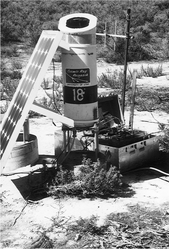
Fig. 9. A flasher station at Dugway Utah. The flasher assembly is inside the white cylinder and is mounted on a concrete post. A steel frame attached to the flasher holds the solar panel. The antenna, control box, and insulated cover box are also shown.
