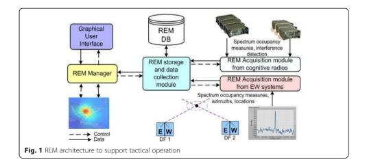
request), and active sensors. REM storage and collection module is an interface between the database, REM acquisition modules, and REM Manager. REM acquisition modules are interfaces to various systems of sensors.
