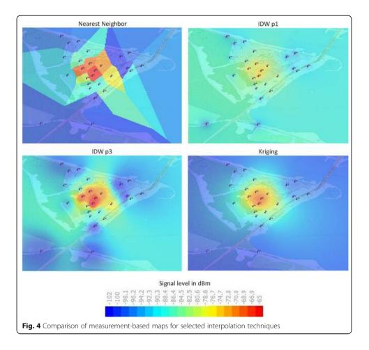
the power p used in the interpolation process. The estimation of the signal strength is quite accurate if the power p is set at 3 or higher and the sensors are deployed densely.
