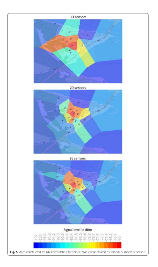
5, 20 sensors and 26 sensors). Moreover, in that case, there are more polygons representing medium level of the emission and they surround the polygons with the highest level. As a result, the map looks more regular. If the number of sensors is very low (Fig. 5, 13 sensors), there are a few polygons that represent medium level of the radio signal. In such a situation, an unnatural effect occurs, namely the polygons exemplifying high signal levels are neighboring with the low-level ones.
