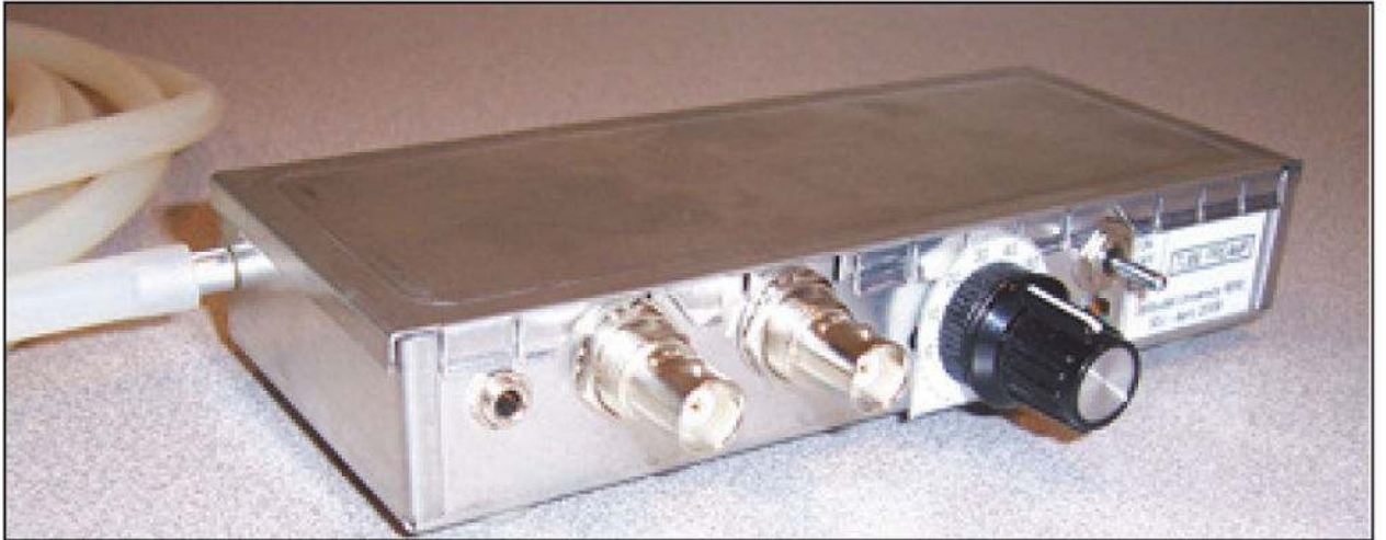
Fig. 7. Switchable gain microphone/amplifier combination. Multiple outputs can feed an A/D converter, an oscilloscope, and computer loudspeakers for audible monitoring.
