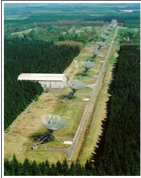
Figure 4.1. Westerbork Synthesis Radio Telescope (WSRT), The Netherlands, operating in selected frequency bands from 110 MHz to 8.6 GHz.
