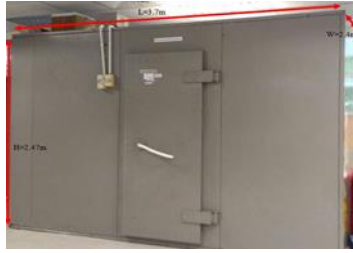
Figure 2. RF-shielded room for indoor measurement setup
