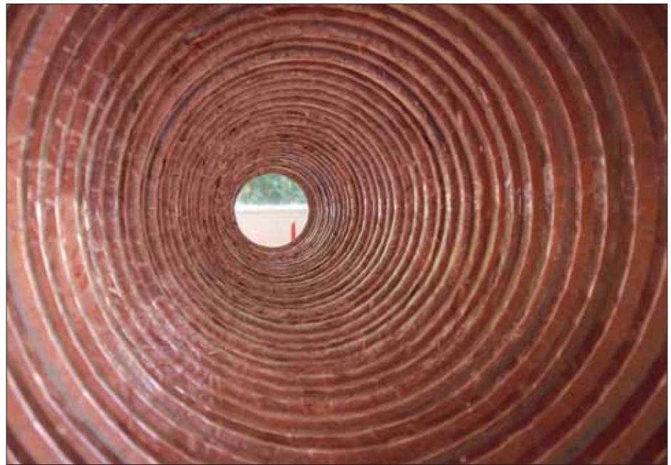
7: Looking into a prototype feed horn for BINGO during construction. It is made from discs of builder's insulating foam, which have aluminium foil on both surfaces; copper tape makes the electrical contact between the top and bottom surfaces when the foam is cut. It all works! (Ian Browne)
