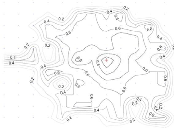
Fig. 4. Contour of PRR from a central node: anisotropy of link quality [Ganesan et al. 2002].
