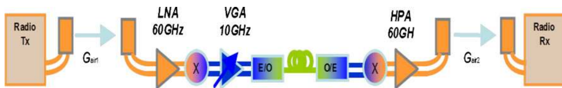
Fig. 5 The system architecture of the ORIGIN demonstrator. Point-to-point variant. Orange parts work at 60 GHz, blue parts at the intermediate frequency and green parts are optical components
