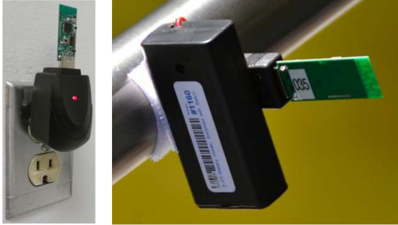
Fig. 7. Two figures of the CC2531 USB dongle node used in the experiments. On the left, a node plugged into an electricity socket through an USB power adapter. On the right, a node powered by two AA batteries.
