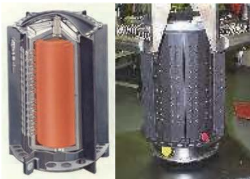
Fig. 19. MHW-RTG. Cutaway view on left. Installation in test fixture on right.
