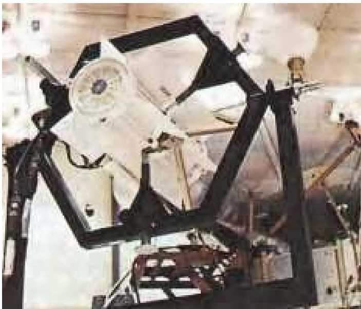
Fig. 12. SNAP-19s installed on Pioneer.
