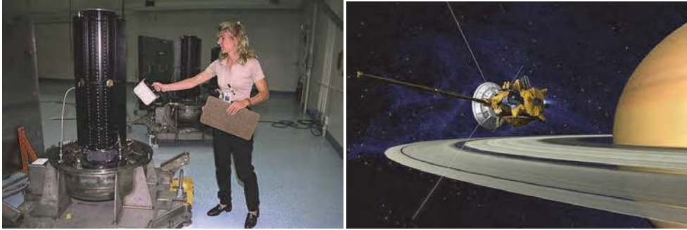
Fig. 25. Cassini spacecraft. Pre-launch checkout of RTG on left. Artist concept of vehicle on right.
