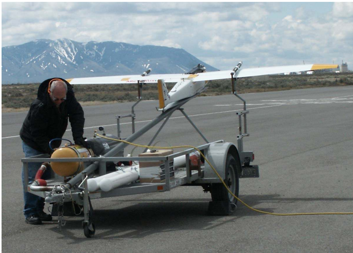
Figure 1. Arcturus T-16 on the catapult launcher at the Idaho National Laboratory (INL) UAV Research Park.
