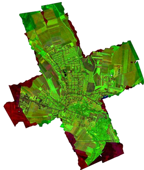
Figure 6. Active multi-wavelength reflectance image estimated from radiometrically calibrated ALS data sets; 532nm (linear scale from 0 (black) to 1 (blue)); 1064nm (linear scale from 0 (black) to 1 (green)) and 1550nm (linear scale from 0 (black) to 1 (red)).
