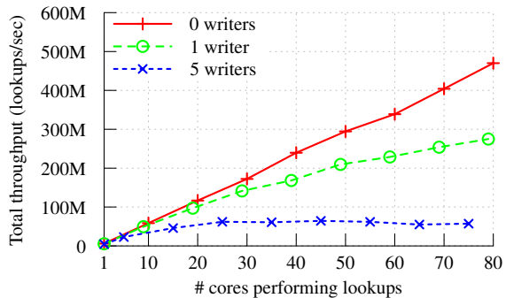
Figure 6: Total throughput of concurrent skip list lookups contending with inserts and deletes.
