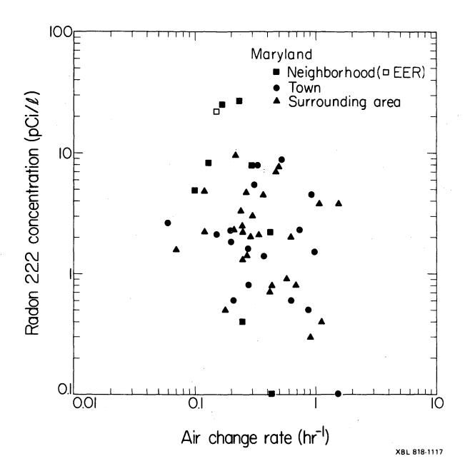
Figure 3. Radon 222 concentrations versus ventilation rates in 52 houses in a community in rural Maryland. The 53rd house (open square), also located in rural Maryland, is one of the energy-efficient houses indicated in Figure 1.
