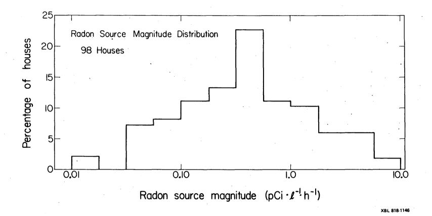
Figure 4. Frequency distribution of radon source magnitudes calculated from the data in Figures 1-3 by taking the product of  $^{22}\mathrm{Rn}$  concentration and ventilation rate.
