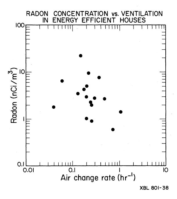
Figure 1. Radon 222 concentrations versus ventilation rates in 17 "energy-efficient" houses, 16 in the United States and one in Canada.
