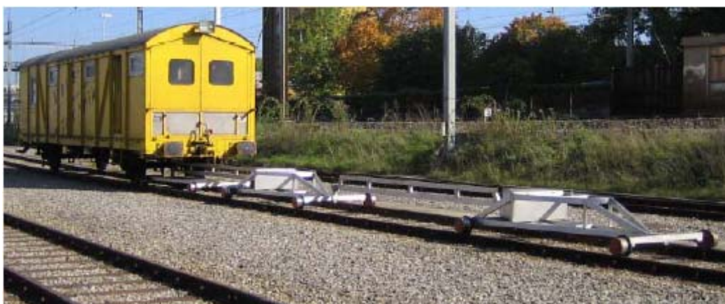
Figure 12. Swiss track stiffness measurement vehicle [62]
