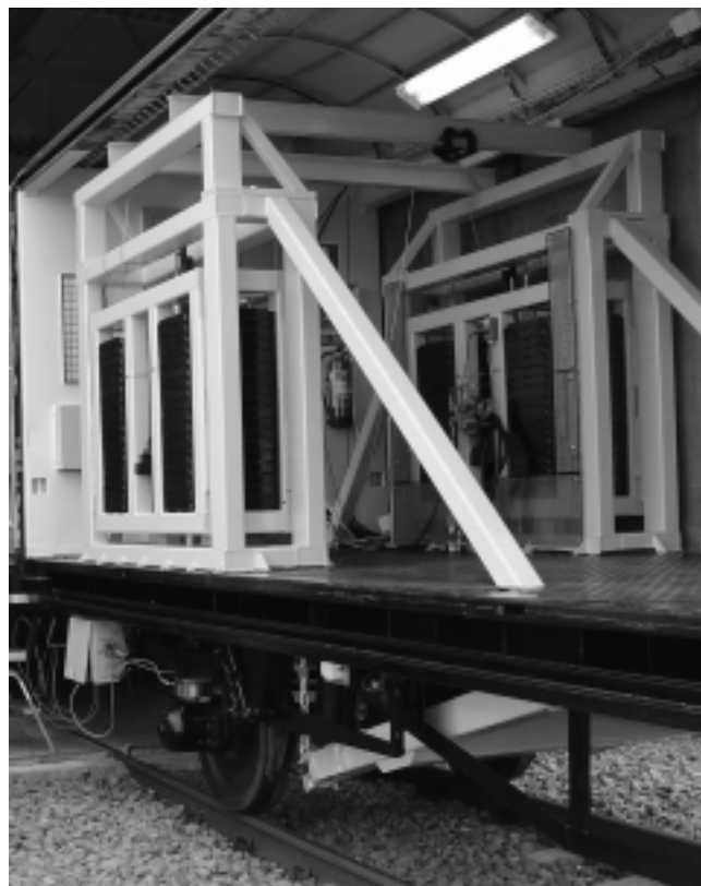
Figure 8. The measurement equipment in the RSMV (vertically moving masses above measuring axle, contained in steel cages).
