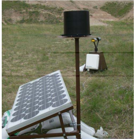
Figure 5. Tipping bucket rain gauge attached to the Solar Panel.
