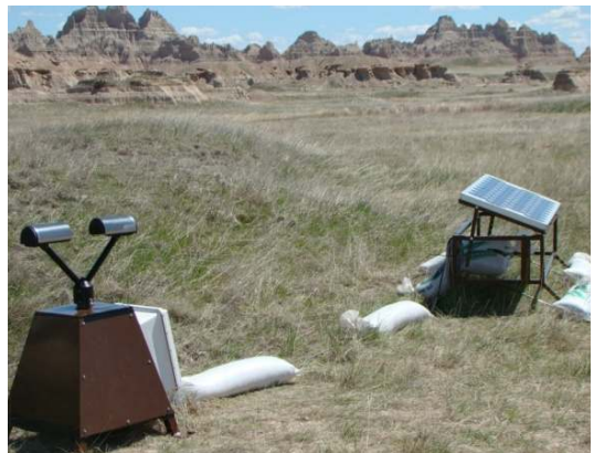
Figure 3. The Parsivel disdrometer and its power source, a solar panel, on location in the North Unit of the BNP.
