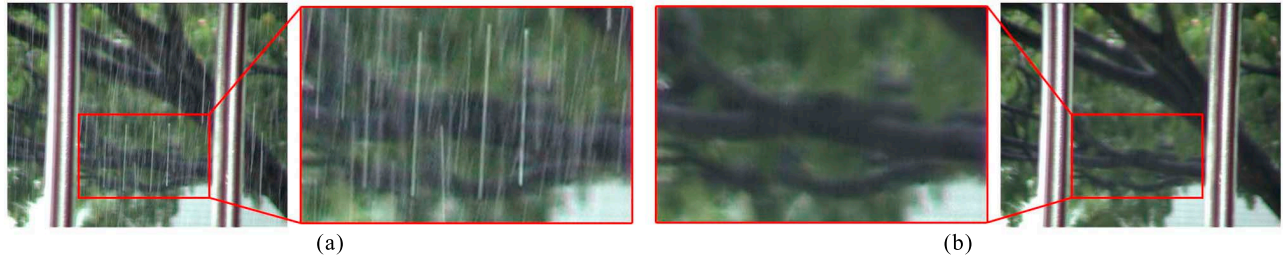
Fig. 5. Rain removal in static scene. (a) A frame in the original video. (b) The derained result.
