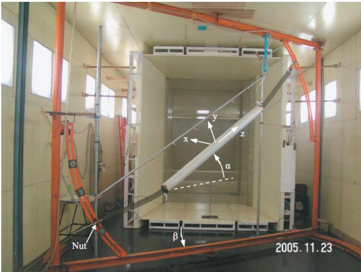
Figure 9.3: New setup for wind-rain-induced cable vibration of [19].
