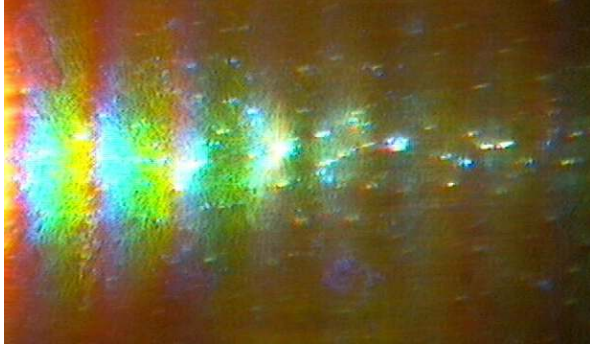
FIG. 6. 'Trapped rainbow' from broadband white light illumination. Colours visibly undergoing cut-off include blue, cyan, green and yellow indicating a wavelength range of \lambda \sim 450\text{nm}-590\text{nm} .
