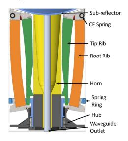
Figure 3: Illustration of key KaRPDA components
