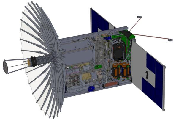
Figure 6. No extra volume is wasted in the final pre-fabrication CAD rendering! The spacecraft is assembled by first installing the integrated radar (left), followed by the bus avionics (right), and finally closing out the system with remaining structure and deployable solar panels.
