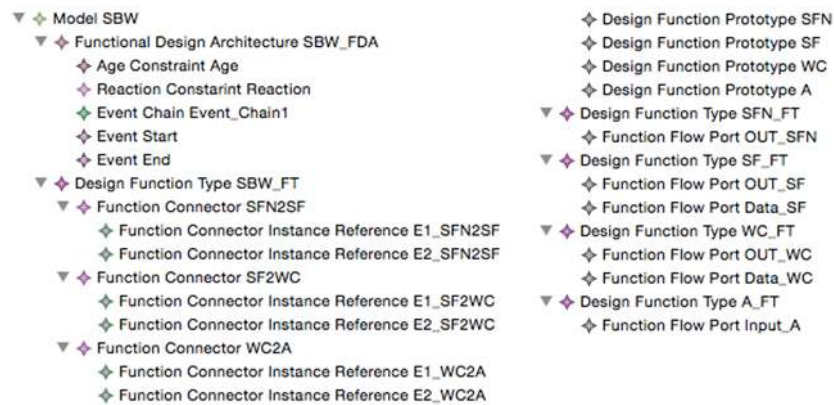
Figure 4.12: Serialized model of the EAST-ADL WC ECU architecture
