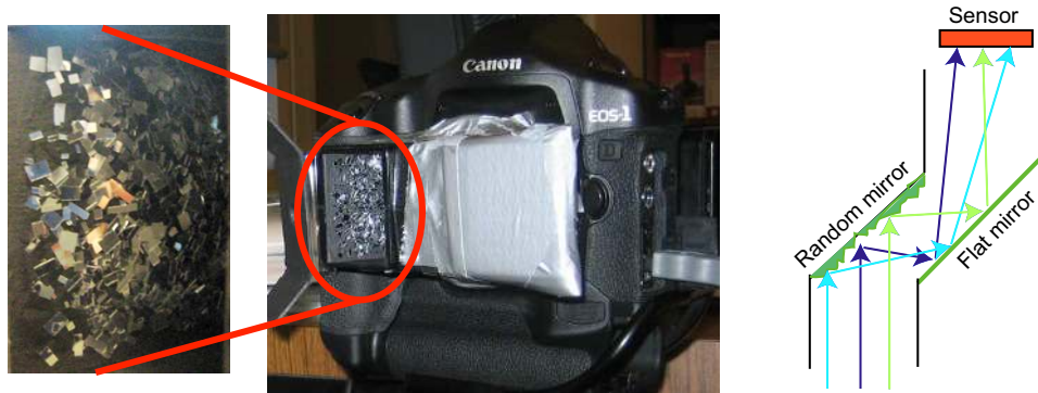
Figure 5: A closeup of the random reflective surface and camera setup used in our experiments. The schematic diagram on the right shows the light path to the sensor.
