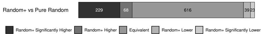
Figure 4. Comparing Random+ performance with Pure Random over the 975 SourceForge classes. (“Random+ Significantly Higher” is the number of classes for which Random+ obtained significantly higher coverage than Pure Random over the 100 runs of the experiment; “Random+ Higher” – the number of class where a higher average coverage was obtained (but not significantly); “Equivalent”, the number of classes where the average coverage level was the same (equal), etc.)
