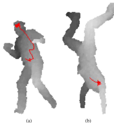
Figure 1. The red lines represents the random tree walks trained to find the head position. The random walk starts from the body center in (a). In (b), the head position is found with fewer steps by starting from the chest, which is much closer than the body center.
