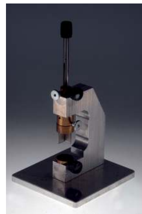
Figure 2. Study-specific device for standardized sectioning of polyvinyl siloxane replicas.
