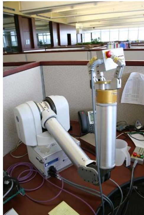
Fig. 1. The Barrett Whole Arm Manipulator (WAM) used for manipulation in populated indoor environments.
