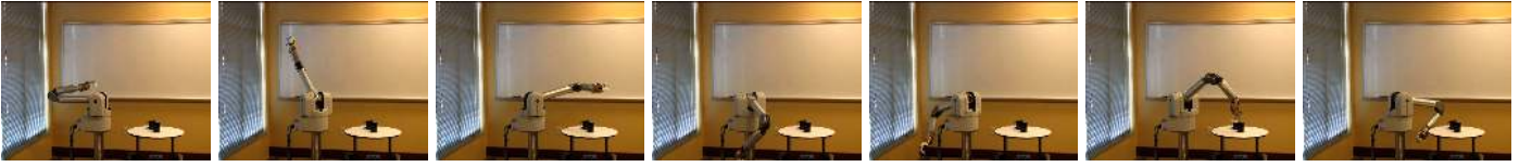
Fig. 6. The example planning problems used in our results. In each case, the manipulator was tasked with planning a path to get its end effector to a desired (x, y, z) location in space. The leftmost image shows the initial arm configuration, the other images show sample arm configurations that satisfied each respective scenario.
