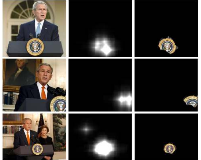
Figure 3: Examples for object localization. The query logo is the same as in Fig. 2. The 1 st column are the original images. The 2 nd column are the voting maps after 200 random partitions. The 3 rd column are the segmentation results with the coefficient \alpha = 5.0 . By comparing the 3 rd row with the first two rows, we can see that this localization strategy is robust to the noisy points which are sparsely distributed in the background.
