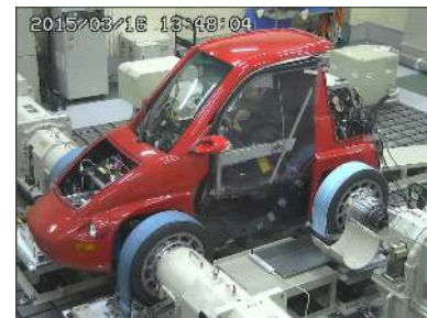
Fig. 1: FPEV2–Kanon on RC–S Bench.
