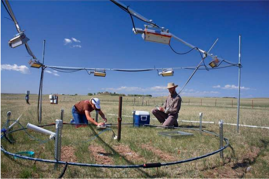
Fig. 4.6 The Prairie Heating and CO 2 Enrichment (PHACE) study located manipulated temperature and CO 2 concentration in C3–C4 shortgrass steppe. Warming was controlled by infrared heaters at the top of each plot, while CO 2 was controlled by emitting gas from the ring at the bottom of the plot (photograph by Sam Cox, (former) USDA-ARS Biological Science Technician, (now) Natural Resource Specialist with Wyoming BLM)
