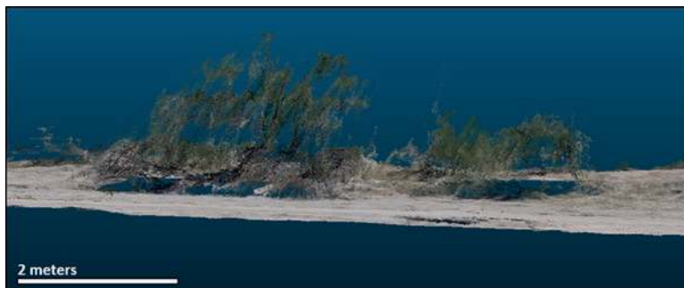
Fig. 16.4 Structure from Motion (SfM) is a new photogrammetric technique that estimates the structure and height of three-dimensional objects from a sequence of two-dimensional images. The SfM algorithm was applied simultaneously to a set of downward-looking and oblique images to produce a point cloud of the canopy structure of creosote ( Larrea tridentata (DC.) Coville) and soil surface elevation below the shrub canopy in the Chihuahuan Desert, New Mexico (J. Gillan, unpublished data)
