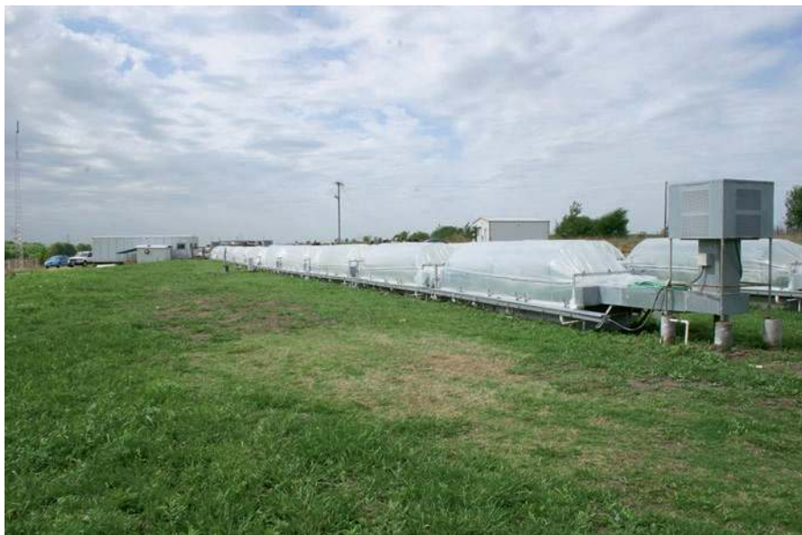
Fig. 4.7 The \text{CO}_2 concentration-gradient study in the tall-grass steppe. Air with an elevated \text{CO}_2 concentration simulating future conditions is introduced at one end and the concentration decreases through photosynthesis as it moves through the tunnel. This allows scientists to examine plant and soil responses ranging from preindustrial to expected levels in 2050 in the same experiment. The experimental infrastructure also allows manipulation of other variables such as soil type (photograph by F.A. Fay)
