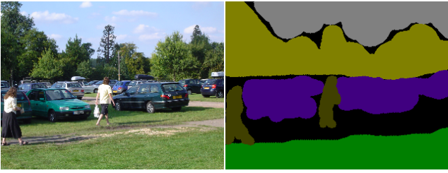
Figure 3: An image from MSRC v2 and the corresponding pixel-level labeling. The classes in this image are ‘sky’, ‘trees’, ‘grass’, ‘body’, and ‘car’. The black regions are ‘void’; we discard void regions.
