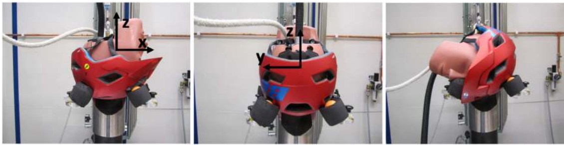
FIGURE 1. The test setup, from left to right Xrot, Yrot and Zrot together with the anatomical coordinate system of the head.
