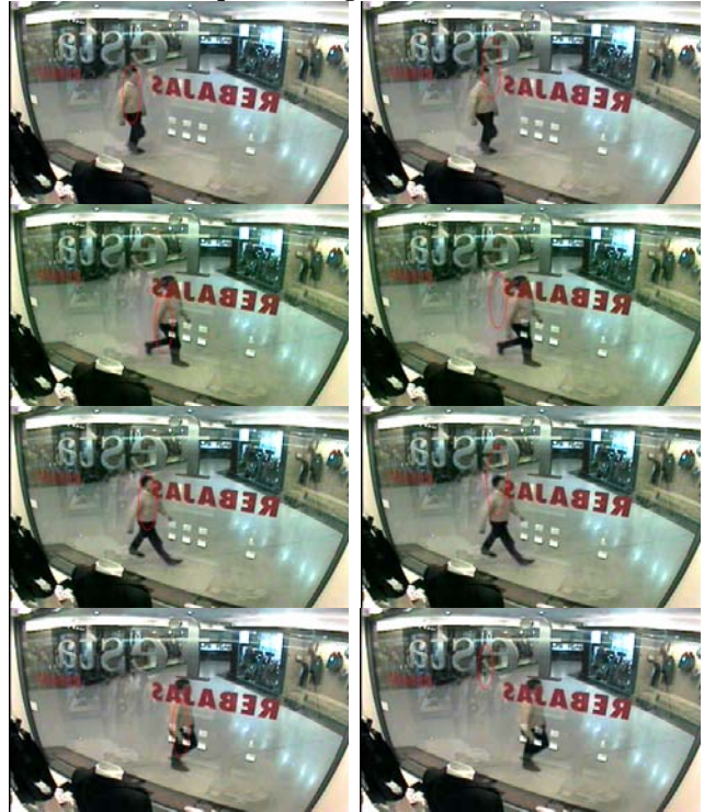
Figure 9. A person is moving in front of a shop window. Left column: RBPF tracker. Right column: PF tracker. The gradient contour is intentionally omitted so that the tracked region is easier to see with the interference of the reflection and the text on the window. In the original sequence (PETS2002 DATASET 1), the frame number is 75,79,84,87.
