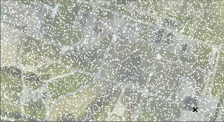
Figure 1.1: Initial particle positions, shown as white dots, spread randomly over the map. The true vehicle position at this time instant is shown as a black cross. Aerial photograph by courtesy of the UAS Technologies Lab, Artificial Intelligence and Integrated Computer Systems Division (AIICS) at the Department of Computer and Information Science (IDA), Linköping University, Linköping, Sweden.
