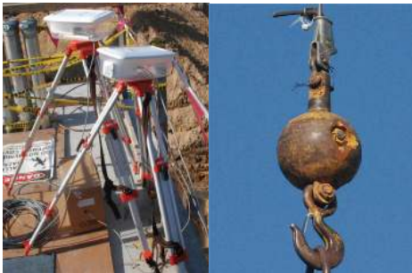
Figure 4 Sensor Field Setup, UWB Tag on Hook
