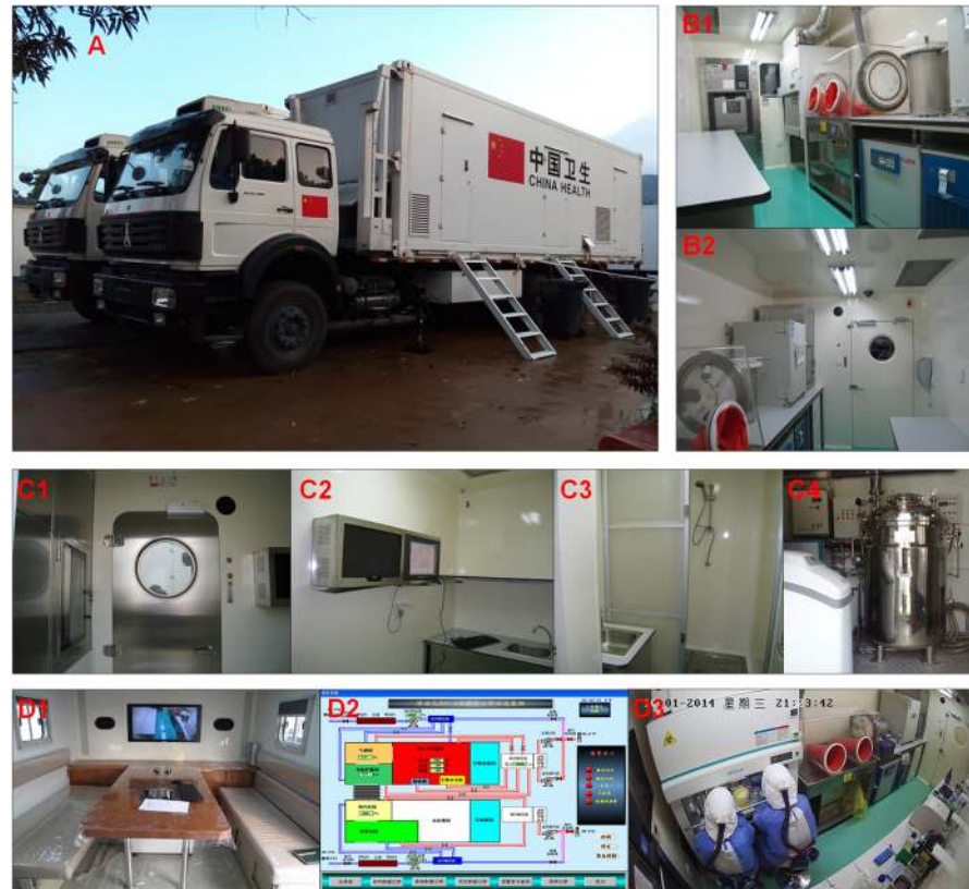
Fig 3. Mobile biosafety level-3 laboratory at its mission in Sierra Leone. (A) Exterior of the mobile biosafety level-3 laboratory. (B) View to the biosafety level-3 laboratory. Two different perspectives (B1 and B2) were shown. (C) View to the auxiliary container. C1) Pass box (left) and expanded-metal door (middle). C2) Monitoring unit and table for experimental preparation. C3) Shower cubicle. C4) Waste treatment room. (D) View to the command container. D1) Room for meeting or for watching monitoring videos. D2) “King View” industry control software. D3) Real-time surveillance video.
