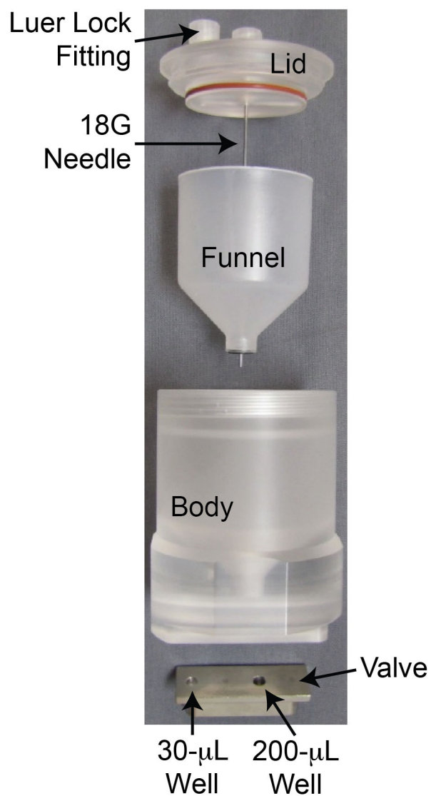
Figure 2. Image of the microbial concentration device. An expanded view of the individual parts of the machined device.
