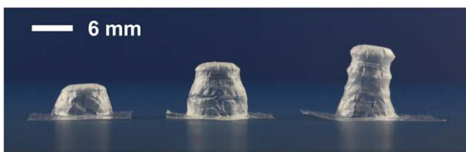
Figure 15. Photographs of bellows (6 mm ID, 9 mm OD, 0.4 mm H , 13.5 μm wall thickness) with 1, 2 and 3 convolutions subjected to pressure just below burst pressure and exhibiting plastic deformation.
