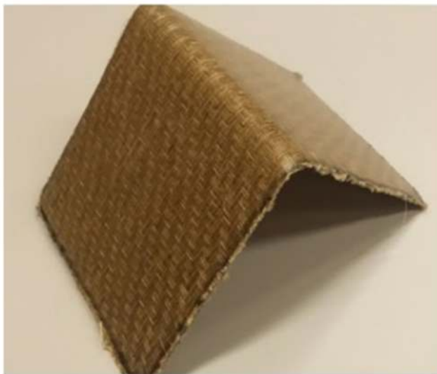
Fig. 6 a Optimized thermal cycle and (b) Composite part manufactured by using the newly optimized process
