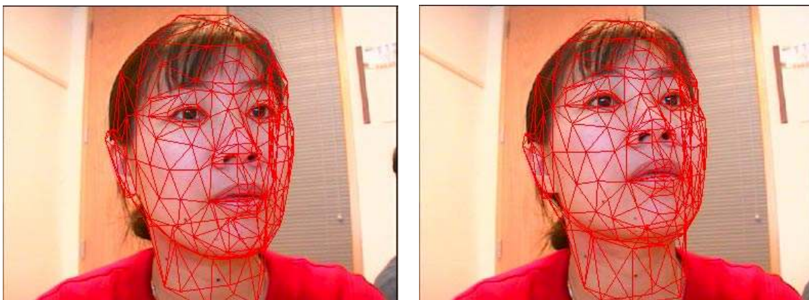
Figure 9: The constructed 3D face mesh is projected back to the two base images.
